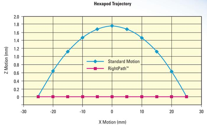
RightPath™ Trajectory Control enables minimal runoff in linear and arc trajectories.
